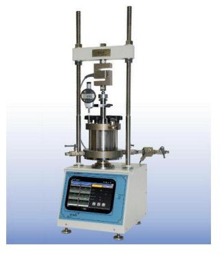
CRS tests are quicker than standard oedometers (typically 24 to 48 hours). They give continuous outputs for Cv and M (= 1/mv) and Void ratio vs vertical effective stress. Running tests at variable rates enables the C-alpha-e to be determined.
